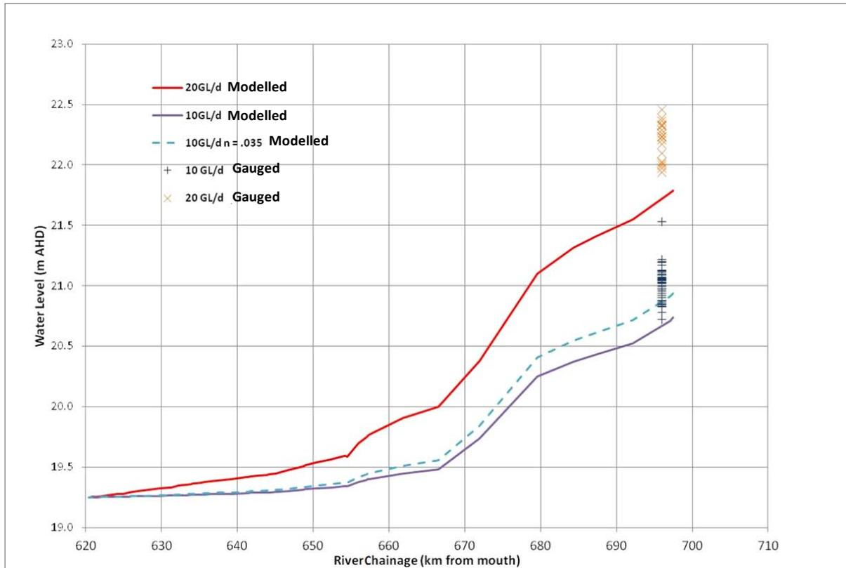
Figure 7: Water level results for calibrating MIKE FLOOD model for Weir Pool 6
