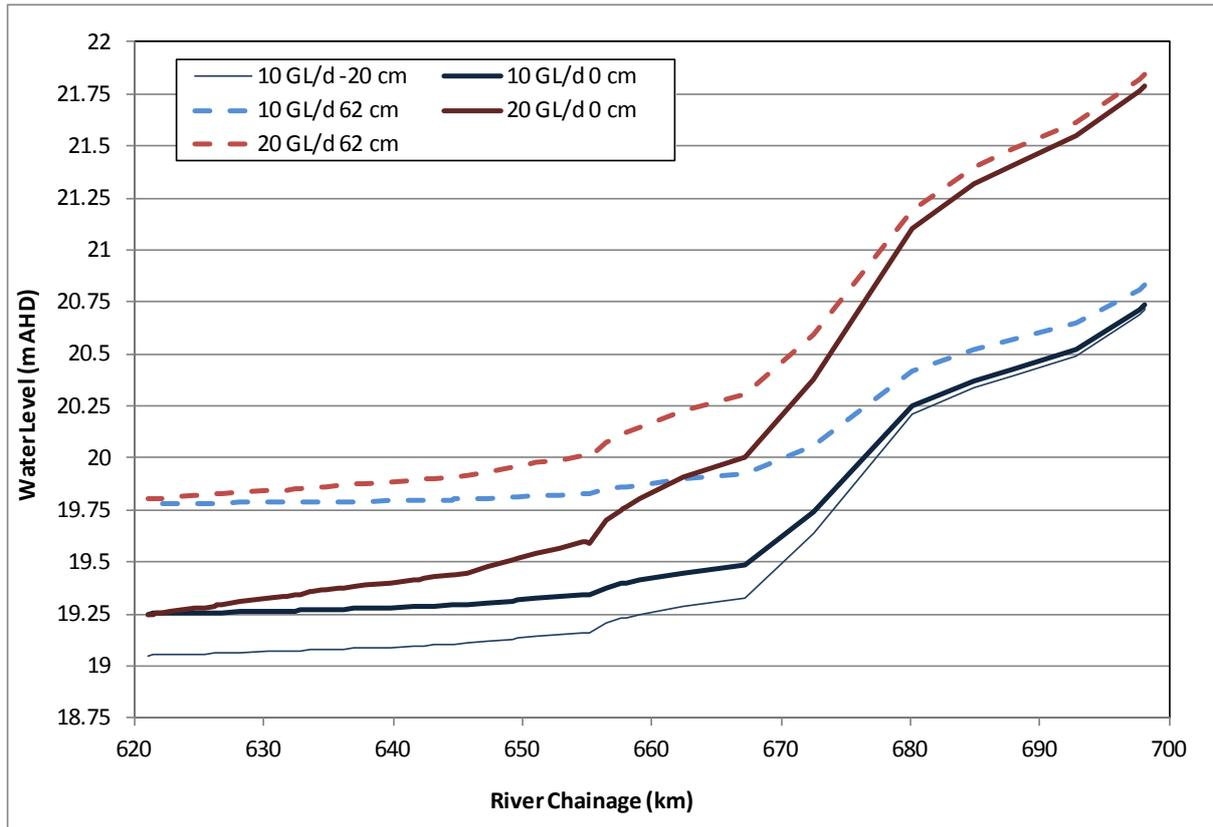
Figure 13: Weir Pool 6 backwater curves for the modelled scenarios
