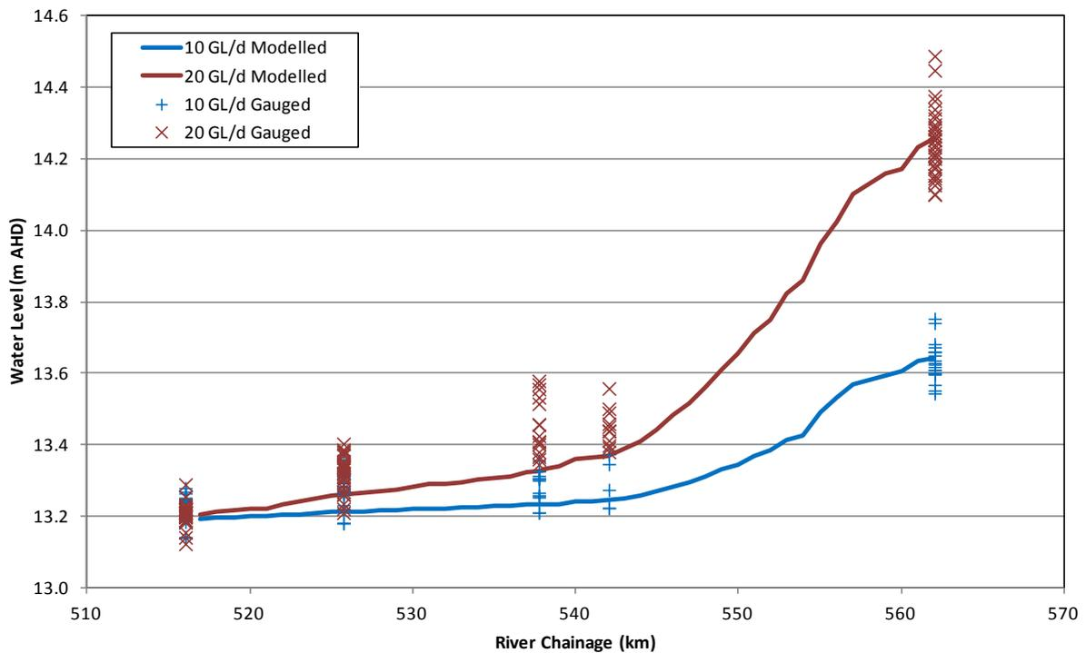
Figure 5: Calibration results of MIKE FLOOD model for Weir Pool 4
