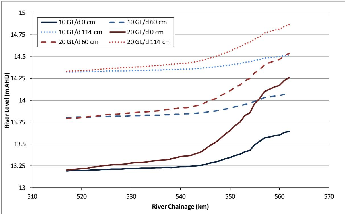
Figure 11: Weir Pool 4 backwater curves for the modelled scenarios
