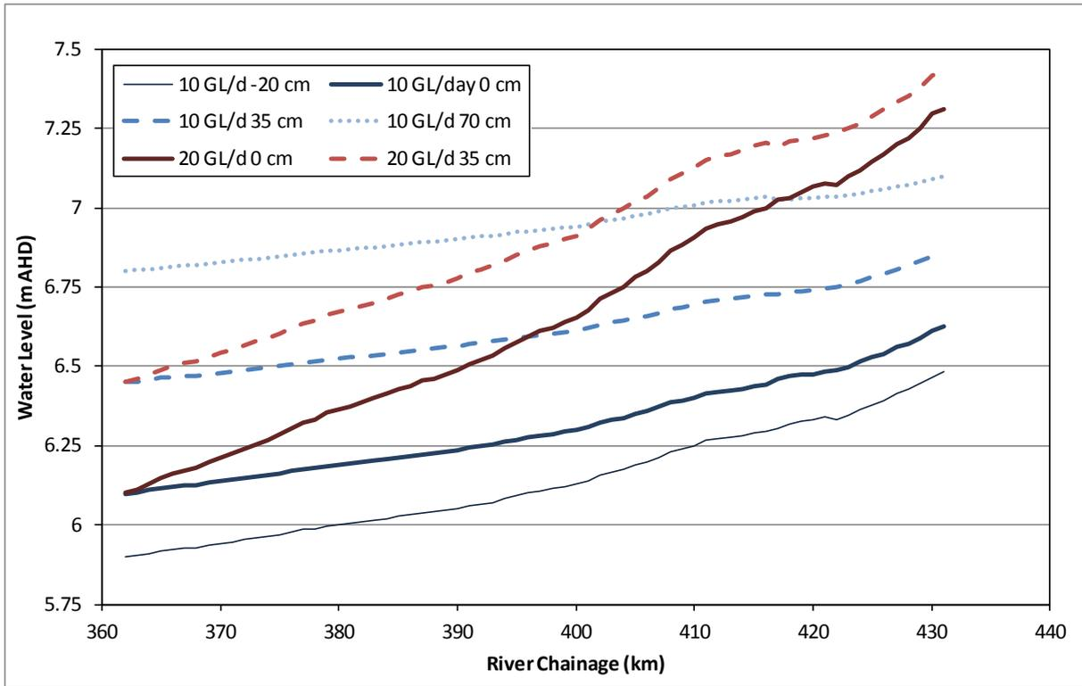
Figure 9: Weir Pool 2 backwater curves for the modelled scenarios
