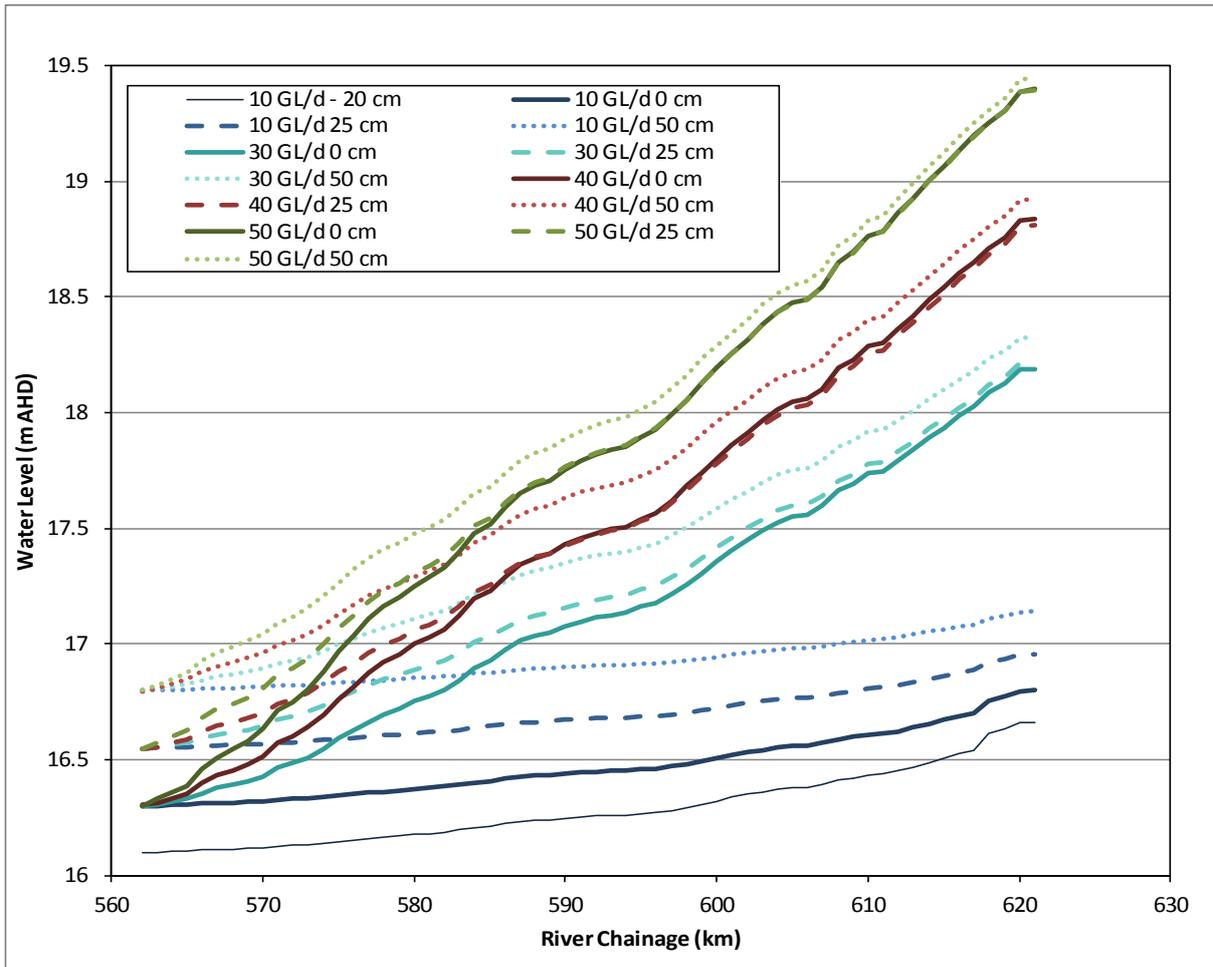
Figure 12: Weir Pool 5 backwater curves for the modelled scenarios
