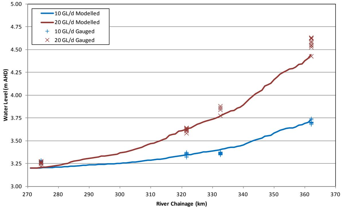
Figure 2: Calibration results of MIKE FLOOD model for Weir Pool 1
