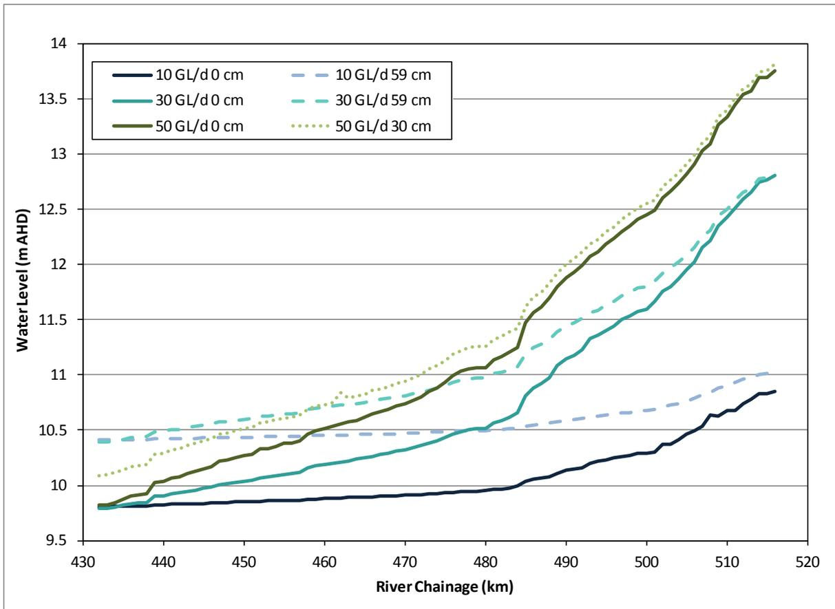
Figure 10: Weir Pool 3 backwater curves for the modelled scenarios
