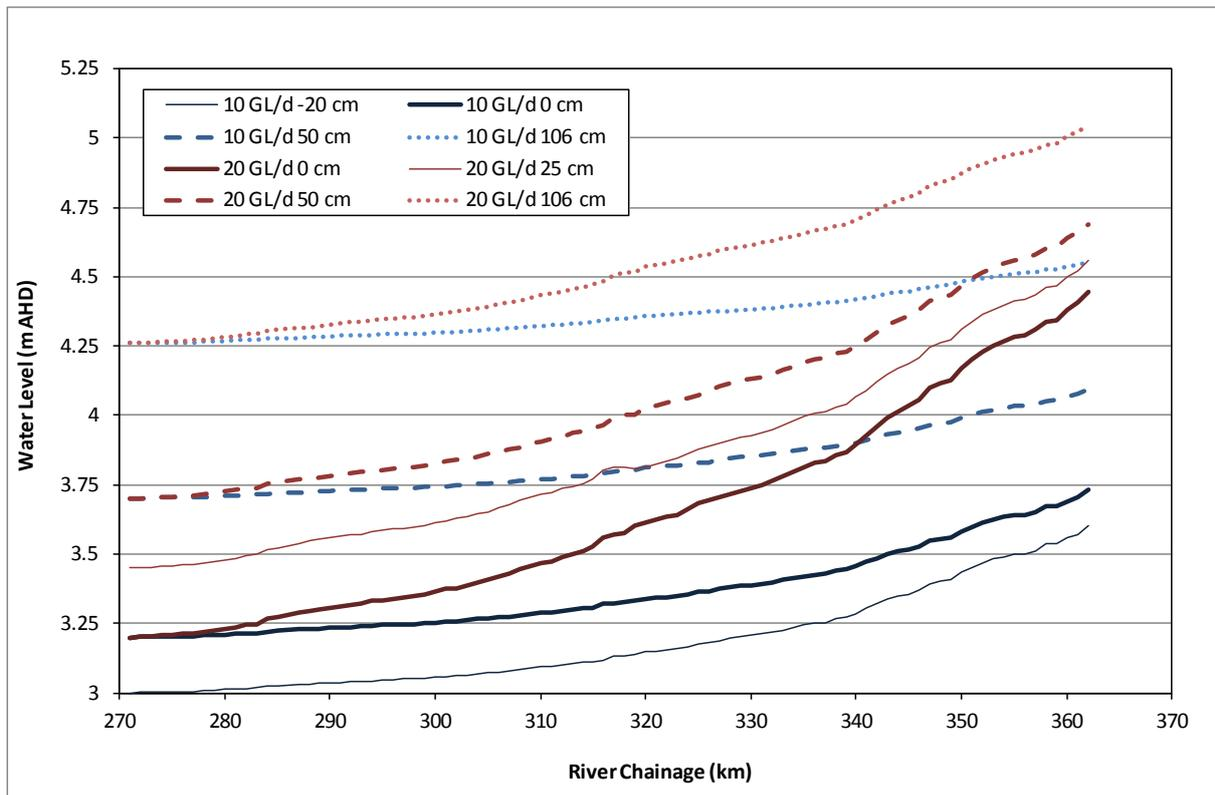
Figure 8: Weir Pool 1 modelled weir manipulation backwater curves for the modelled scenarios
