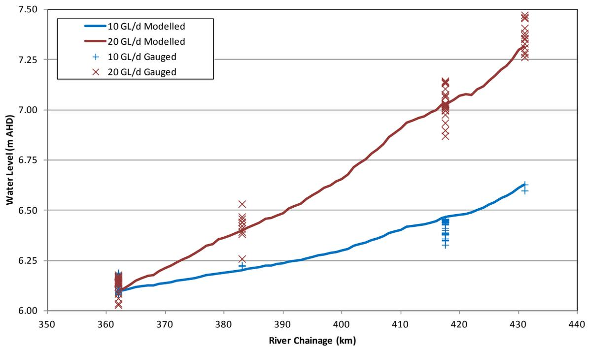
Figure 3: Calibration results of MIKE FLOOD model for Weir Pool 2
