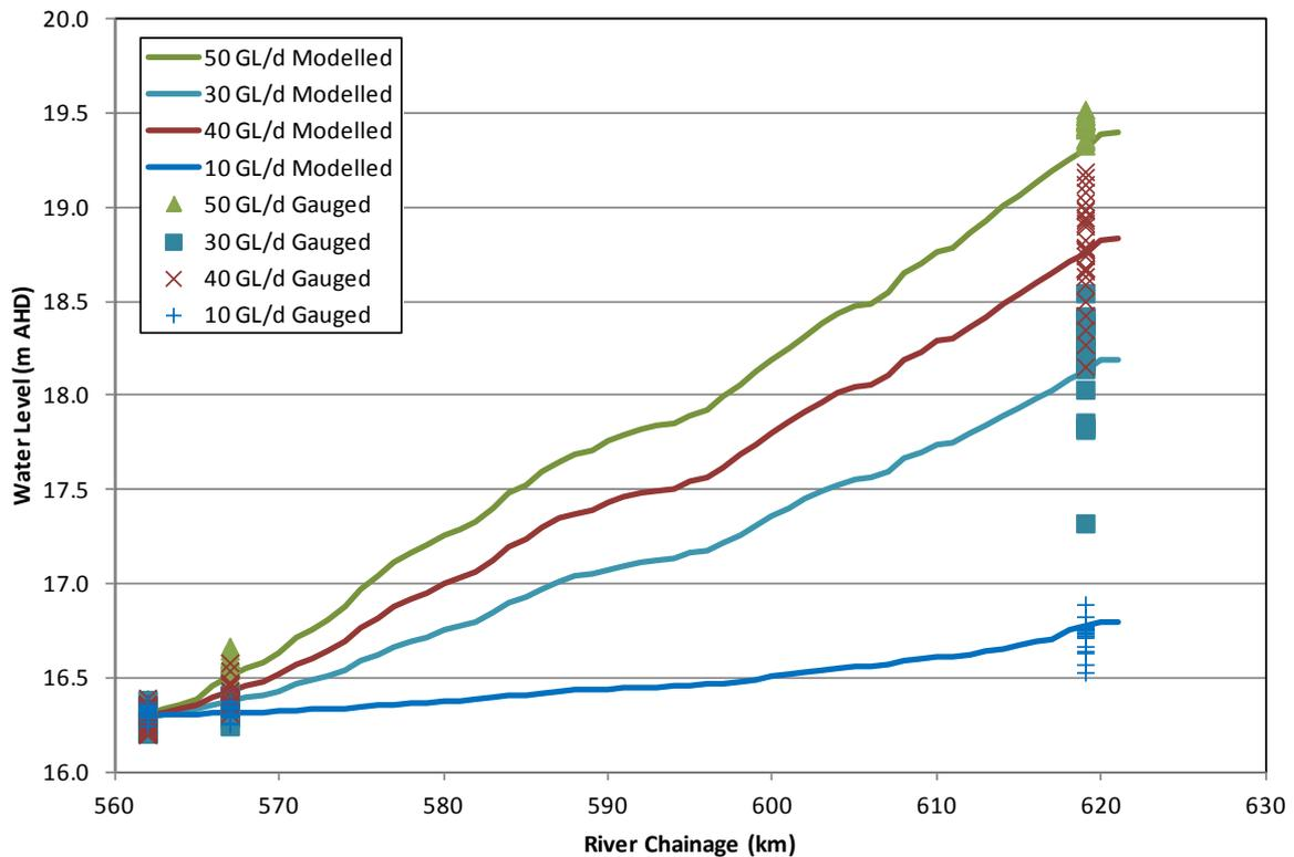
Figure 6: Calibration results of MIKE FLOOD model for Weir Pool 5
